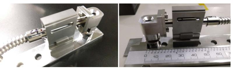
High precision hexabundle ferule, magnet casings and coupling components manufactured to align optical fibre bundles accurately to galaxies on the Hector field plate. Machining by Nicholas Hacko Watchmakers/NHmicro. Credit: Prof Julia Bryant, Astralis-USyd.
