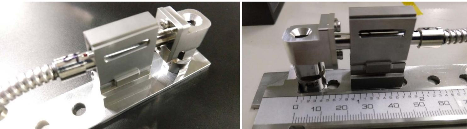
High precision hexabundle ferule, magnet casings and coupling components manufactured to align optical fibre bundles accurately to galaxies on the Hector field plate. Machining by Nicholas Hacko Watchmakers/NHmicro. Credit: Prof Julia Bryant, Astralis-USyd.
