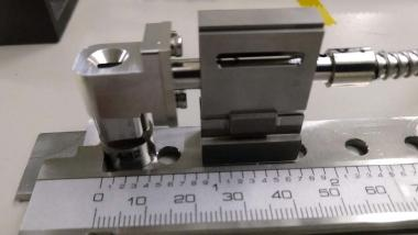
High precision hexabundle ferule, magnet casings and coupling components manufactured to align optical fibre bundles accurately to galaxies on the Hector field plate. Machining by Nicholas Hacko Watchmakers/NHmicro. Credit: Prof Julia Bryant, Astralis-USyd.
