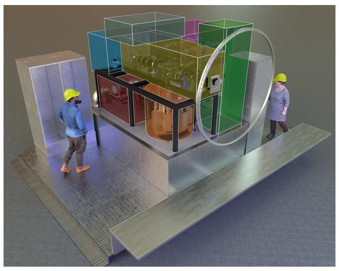
A rendering of MAVIS on ESO's VLT/UT4 Nasmyth platform (placed on the side of the telescope) highlighting the main modules: yellow – adaptive optics module; orange – laser guide star wavefront sensor; red – natural guide star wavefront sensor; blue (behind) – imager; fuchsia – spectrograph; green – calibration unit. Credit: ESO/MAVIS Consortium/L. Calçada.
