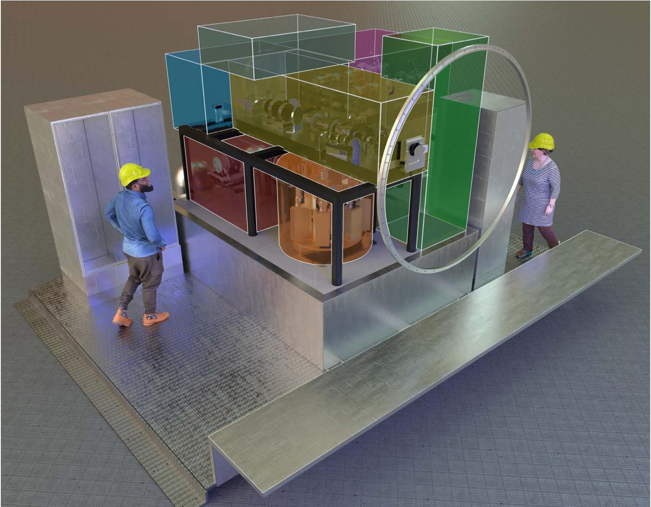
A rendering of MAVIS on ESO's VLT/UT4 Nasmyth platform (placed on the side of the telescope) highlighting the main modules: yellow – adaptive optics module; orange – laser guide star wavefront sensor; red – natural guide star wavefront sensor; blue (behind) – imager; fuchsia – spectrograph; green – calibration unit. Credit: ESO/MAVIS Consortium/L. Calçada.
