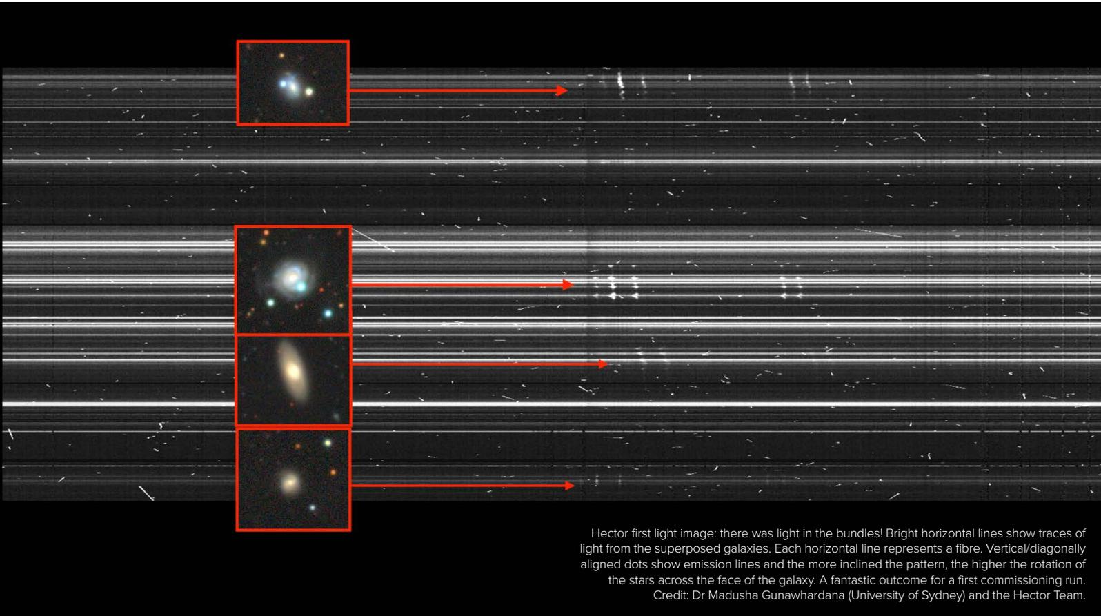
Hector first light image: there was light in the bundles! Bright horizontal lines show traces of light from the superposed galaxies. Each horizontal line represents a fibre. Vertical/diagonally aligned dots show emission lines and the more inclined the pattern, the higher the rotation of the stars across the face of the galaxy. A fantastic outcome for a first commissioning run. Credit: Dr Madusha Gunawardana (University of Sydney) and the Hector Team.
